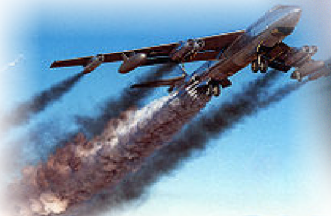
B -47, Stratojet with Rocket - assisted Take Off
